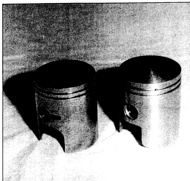
The Suzuki GT250 piston on the left has a narrower rear inlet skirt; modified Arrow piston on the right.
