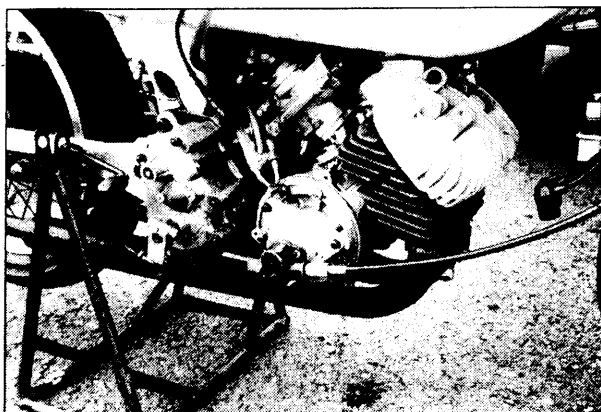
View of the alternator side shows a complex splayed manifold and engine mounts welded to the cylinder heads.
